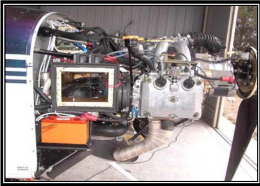
#9 COOLING DUCT FANS
